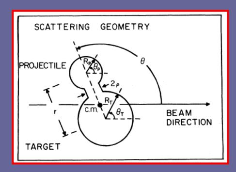
$$\left[\frac{d}{dt}\frac{\partial}{\partial \dot{q}_{i}} - \frac{\partial}{\partial q_{i}}\right]L = -\frac{\partial}{\partial \dot{q}_{i}}F, \quad q_{i} \in \{r, \theta, \theta_{p}, \theta_{T}\}$$
